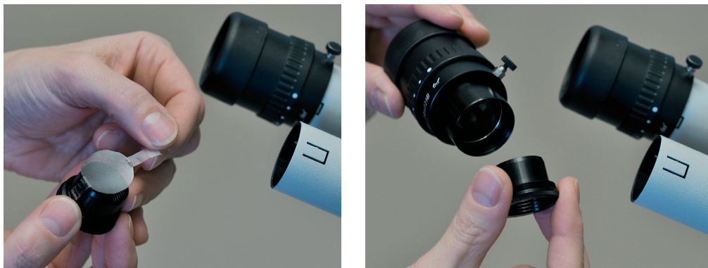
Figs. 2 & 3: Cutting of Film Discs and Their Attachment to Microscope Eyepiece
