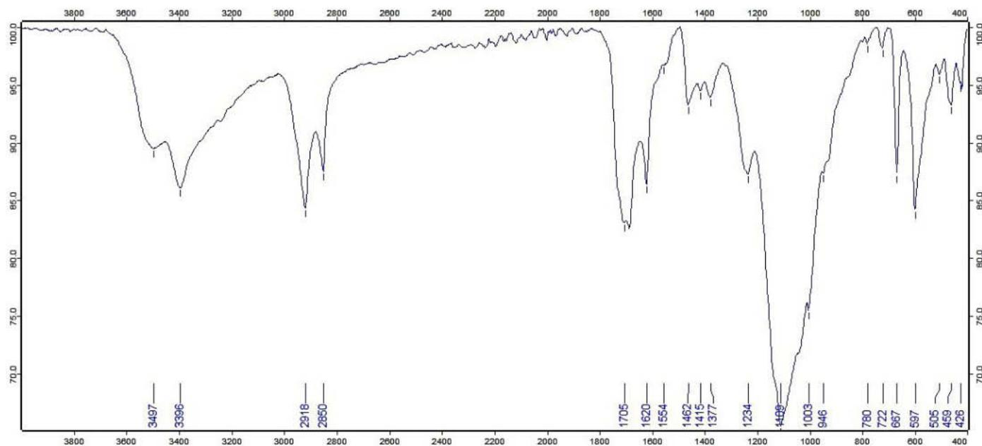
Fig. 8. FTIR results of varnish.
