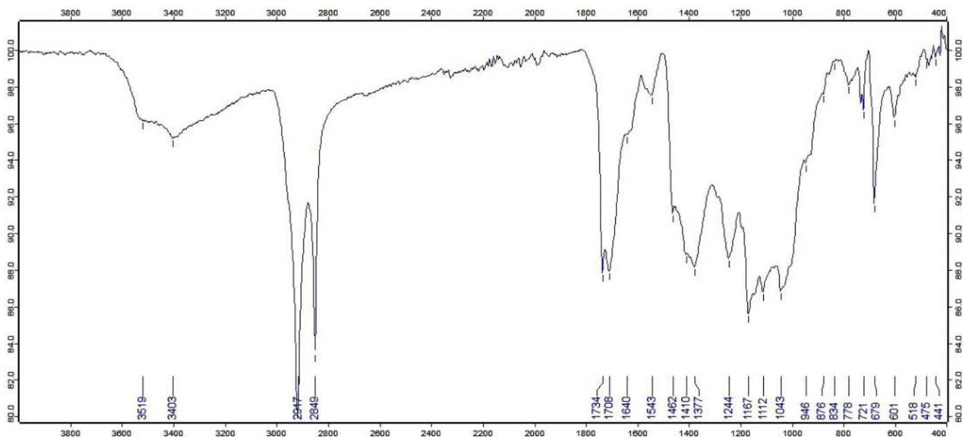
Fig.15. FTIR spectrum of the white painted layer.
