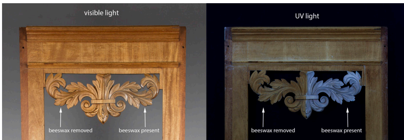
Fig. 6. Part of the mahogany case showing the restoration coating of beeswax in normal light and UV light.
