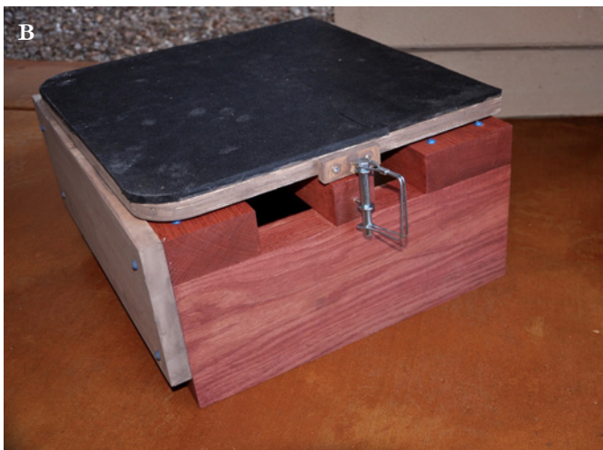
Fig. 9. (A) New base for sculpture with lazy Susan attachment. (B) New base with top and locking pin, fully assembled.
