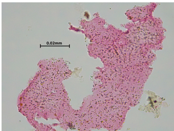
Fig. 16. PPL photomicrograph of dispersed finish media. The binding media appears dyed, and small particles of pigment and dirt are present.
