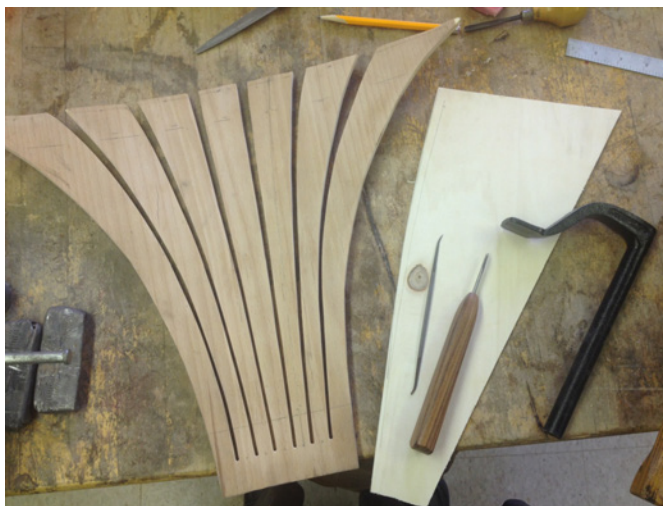
Fig. 20. A scorp and riffler were used to engrave the splats of the fanned back splat.
