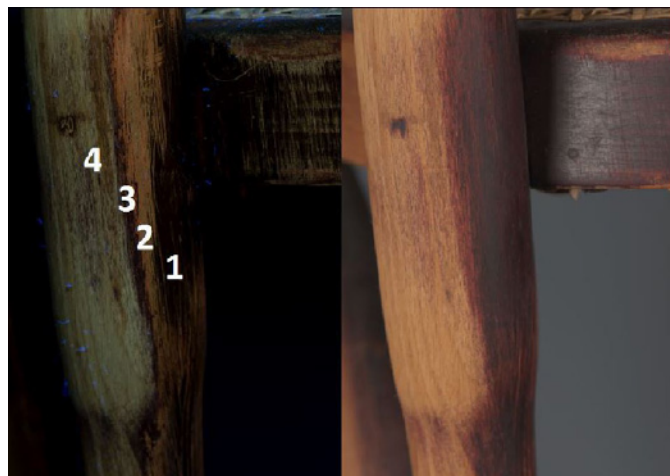
Fig. 10. Sanded proper right stile, comparison of normal illumination (left) and UVA-Vis (right). (1) Exposed wood. (2) First layer(s) of nearly nonfluorescent finish. (3) Second layer(s) of bright orange-yellow finish. (4) Top layer(s) of nearly nonfluorescent finish.
