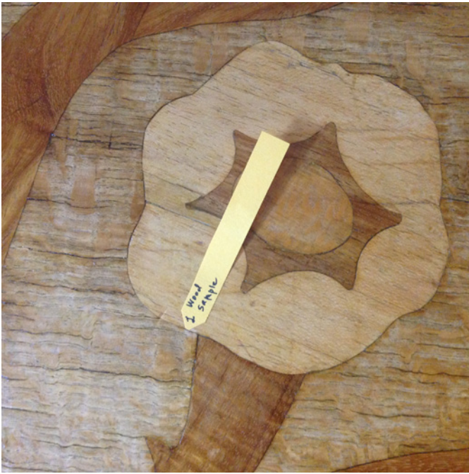
Fig. 14. Sampling location for collection of thin section from the veneer for microscopic wood identification. Flat-cut oak veneer provides radial section for microscopic investigation.
