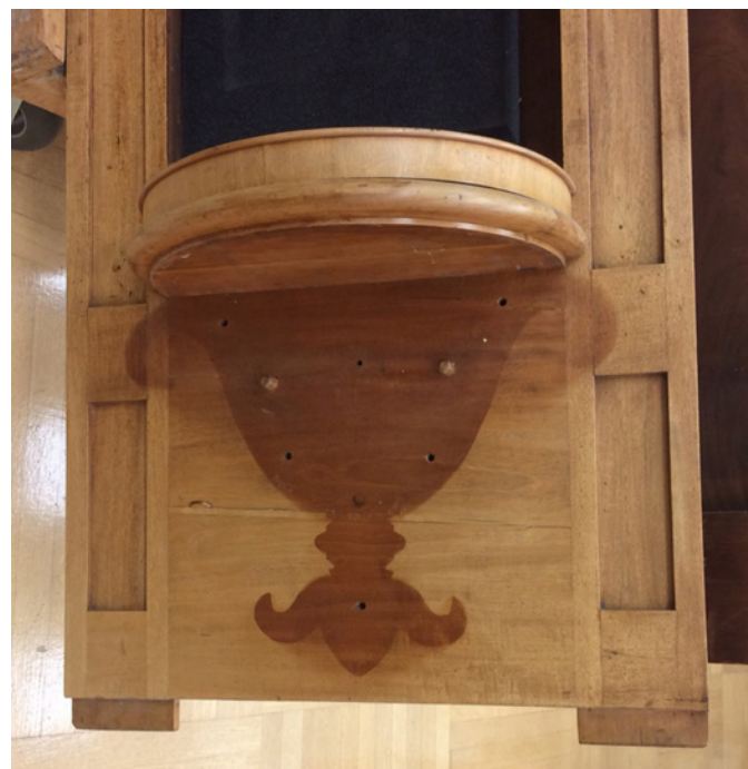
Fig. 5. Part of the mahogany case showing the original color in an area protected from light by a decorative element and the faded color in unprotected areas.
