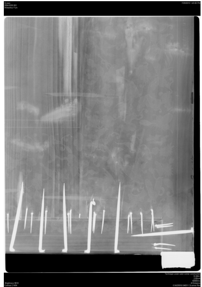
Fig. 3. X-radiograph of one of the panels of screen 2004.0030.002. The long nails used to attach to top and bottom boards can be seen, as well as the wooden dowels that peg the vertical boards together. Courtesy of the Winterthur Museum.
