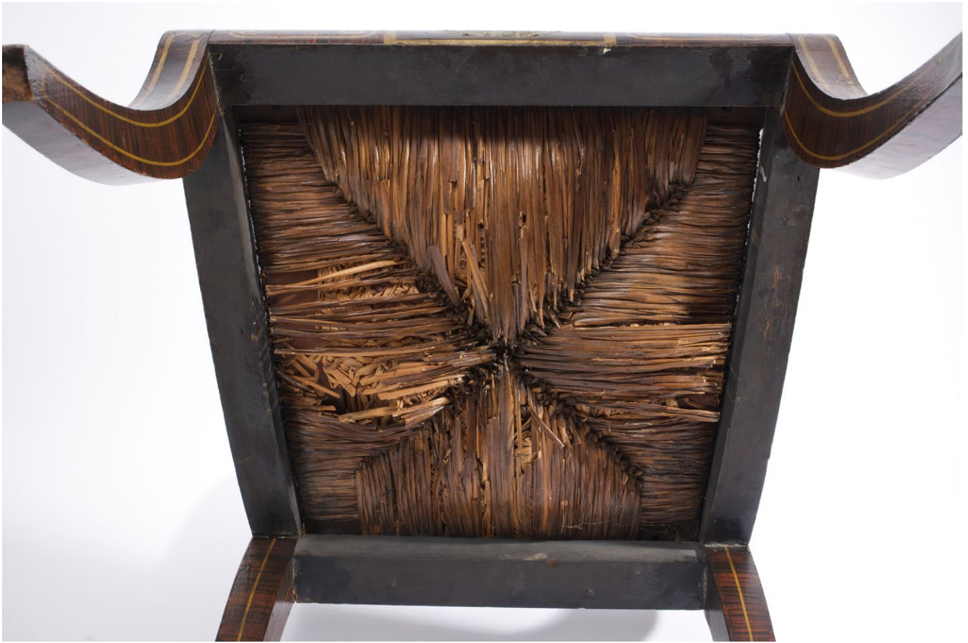
Fig. 5. Failing rush below chair seat. Courtesy of Arthur Evans ©
