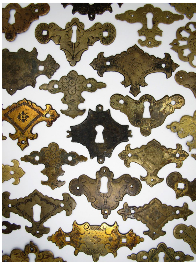
Fig. 1. A group of brass back plates and escutcheons made between 1700 and approximately 1745. These objects were sand-cast with a beveled edge on one side. The surface of each plate was refined with a triangular scraper and decorated by hand with chasing and matting tools and occasionally, engraving tools.
