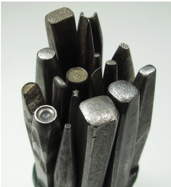
Fig. 4. Detail of chasing and matting tools: The designs and patterns were stamped into the brass after casting.
