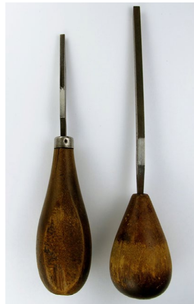
Fig. 5. Engraving liners: White watercolor highlights the pattern of parallel lines that will be engraved by the tool.
