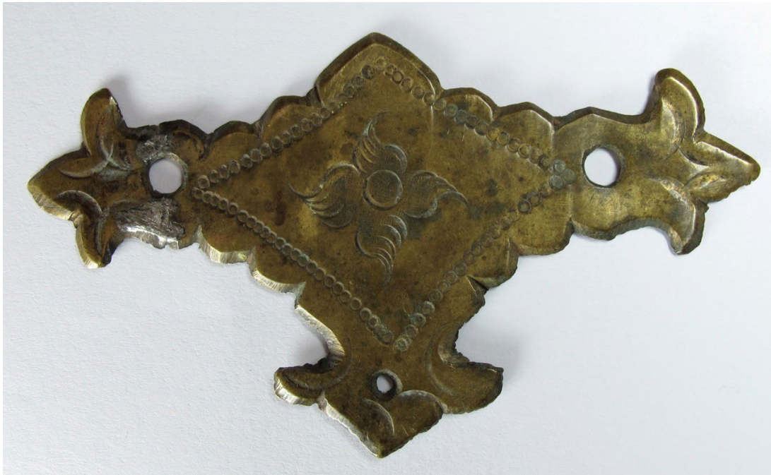
Fig. 3. The beautiful waves on the face of this back plate were created when the triangular scraper was used to remove the rough surface inherent to the sand casting process. The delicate chatter lines on the beveled edges of 18th-century cast brasses were made with hand-files or sometimes with a triangular scraper.
