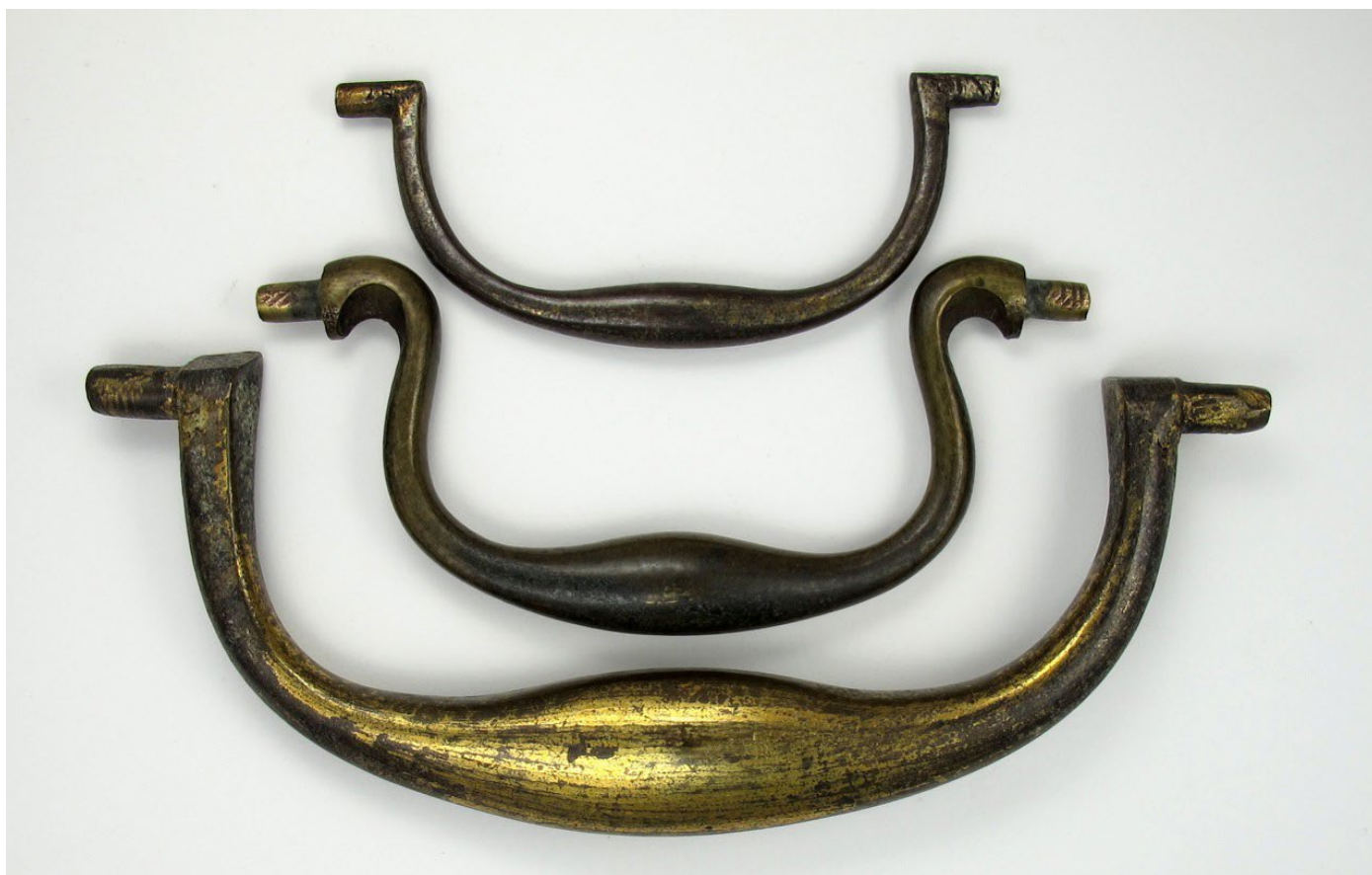
Fig.10. Note the numbers and the Roman numerals on the ends of the top two bails. These markings are for size or part identification. (The bails with the Roman numerals are possibly by John Clarke and Son of Birmingham). The lovely form of the large lift handle looks as though it was sculpted by a triangular scraper and a burnisher. Please note the beautiful lines made by these tools. It is doubtful that similar lines would be found on a reproduction bail. This lift handle feels like silk.
