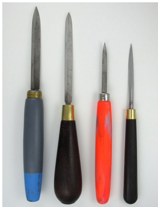
Fig. 2. Triangular scrapers; the small one on the right is a sail maker's needle that has been sharpened and fit into a handle.
