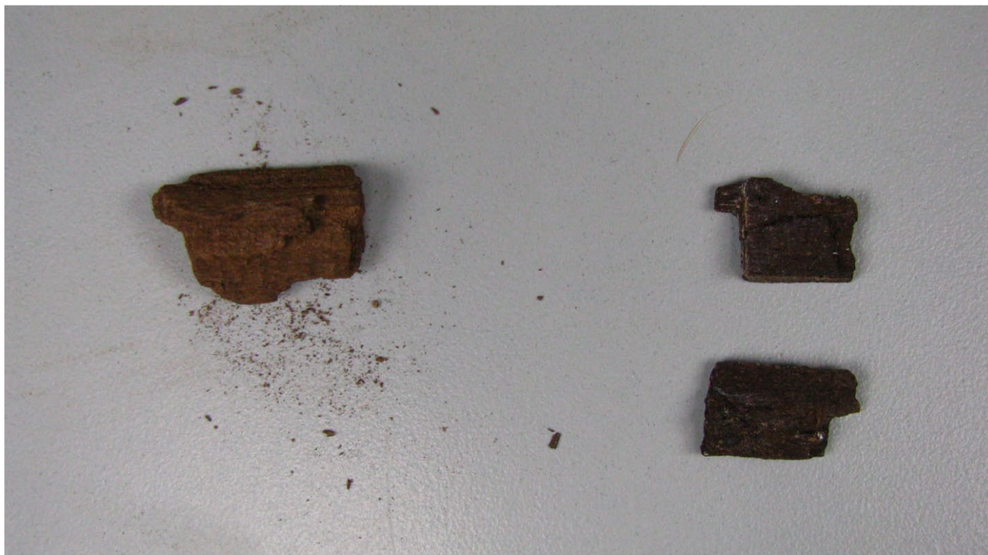
Fig. 3. Untreated (left) and TEOS treated (right) samples. The consolidated sample was treated with seven drip applications of Remmers KSE 300, applied at one-day intervals.
