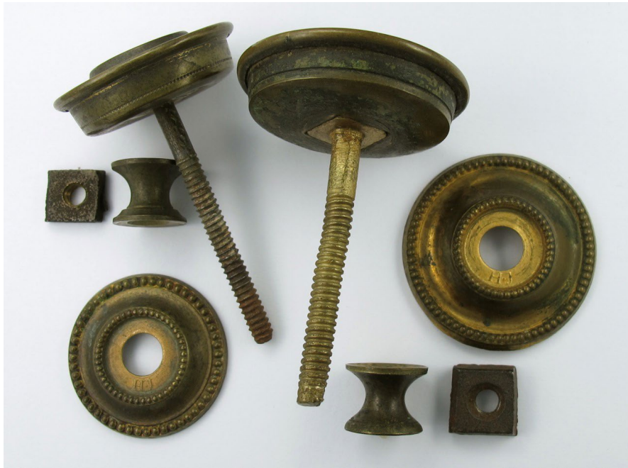
Fig.12. Examples of hollow pressed brass knobs made by Thomas Hands and William Jenkins illustrating their construction techniques. Note the HJ maker's mark in each knob back plate. The spool-shaped base and the back plate are secured to the knob with the large square iron nut. This iron nut screws up underneath the pressed back plate.
