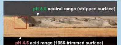
Fig. 4 Section of pine newel post trimmed for the 1956 installation at The Met
