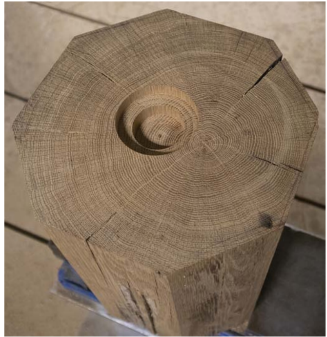
Fig. 13. Oak block with milled cavity for mount. The center of the finial was placed away from the pith as much as possible. (© The Metropolitan Museum of Art)
