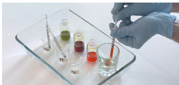
Figure 1. Mixing the sensitizer using 2 parts of the iron solution, 1 part of the platinum solution, and 1 part of the palladium solution.
