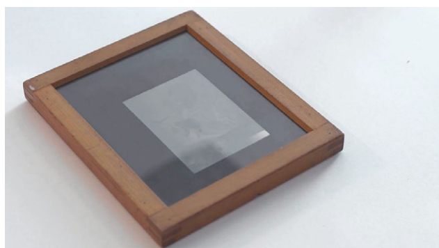
3d. The printing frame assembly is shown ready for exposure.
