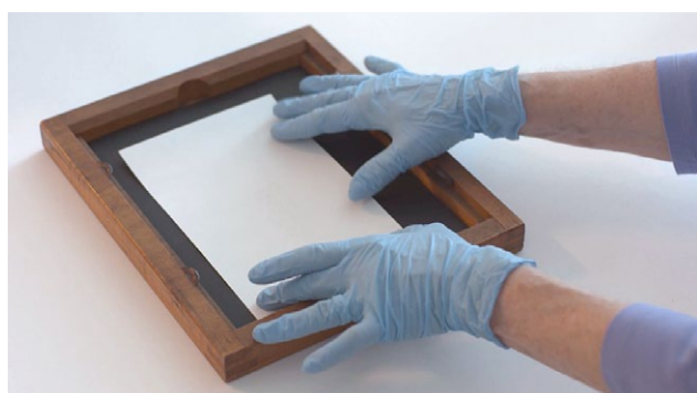
3b. The sensitized side of the paper is placed in direct contact with the negative.
