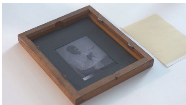
3a. The negative is placed in a wooden printing frame, emulsion up, against the glass, along with a black paper mask.
