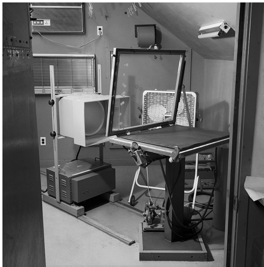
Figure 9. One of the plate exposing rooms in Lab A, c. 1986, showing a 4000 watt pulsed xenon arc printing lamp at left and vacuum frame. A box fan was used to reduce heat buildup of the vacuum frame glass. The sensitized plate was placed on the rubber platen, the film positioned on the plate's register strip, the glass closed, and a vacuum drawn to create perfect contact. The vacuum frame was then rotated into a vertical position for exposure to the light of the xenon arc lamp. © The Irving Penn Foundation.
