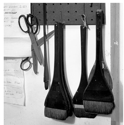
Figure 16. Sensitizing brushes hanging from pegboard above the coating table in Lab A, c. 1986. © The Irving Penn Foundation.
