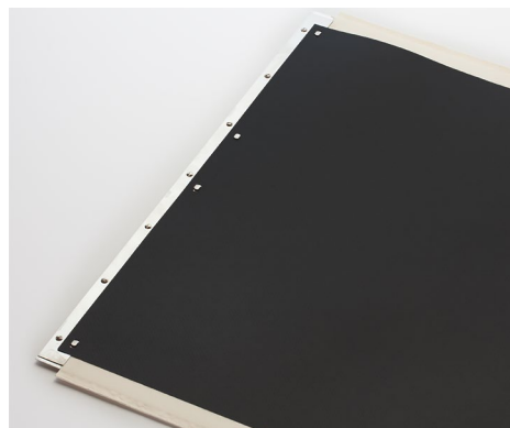
13e. Register strip bolted to the sensitized plate and the punched film placed on the registration pins.
