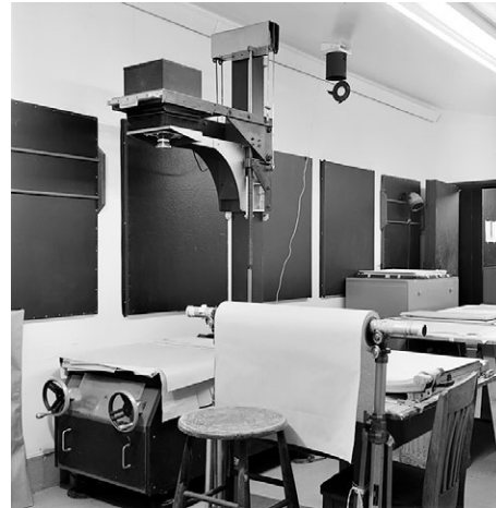
Figure 10. Lab B's film exposing and plate-making room, c. 1986. A roll of the heat-set film Surlyn, in the foreground, is positioned to mount the paper to the aluminum sheets. The custom-built 8 × 10 inch enlarger used to make enlarged interpositives is at left. A simple point-light source, which hangs from the ceiling just behind the enlarger, was used for exposing full-scale negatives and masks by contact. © The Irving Penn Foundation.
