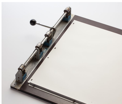
Figure 13. Irving Penn's registration system, photographed in 2017. For clarity of illustration, paper is shown in lieu of film.
