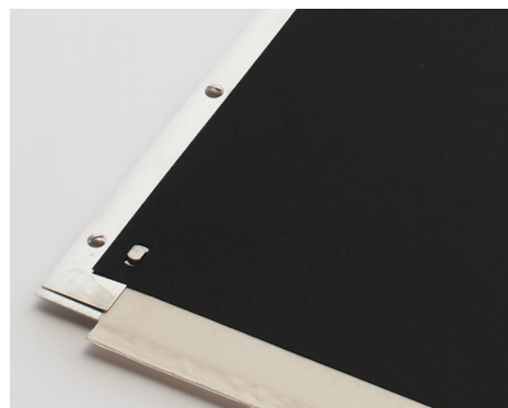
13f. Detail of film in place on the sensitized plate, ready for exposure in vacuum frame.
