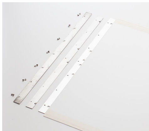
13c. Stainless steel register strips and punched plate. The top edge of the plate shows the exposed aluminum with holes that correspond to the round pins on the back of the register strips (large holes) and bolts (small holes) that held the register strips to the plate.
