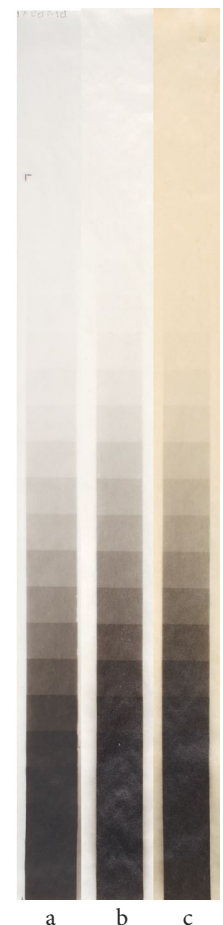
Figure 18. Platinum step-tablets on vegetable parchment paper made by the Photograph Conservation Department, National Gallery of Art. (a) Uncoated print before aging. (b) Print coated with Strand's varnish before aging. (c) Print coated with Strand's varnish after artificial aging.
