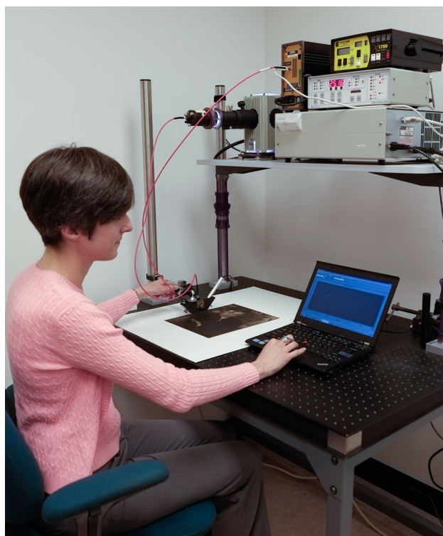
Figure 1. Conservation scientist Joan M. Walker operating the microfading tester at the National Gallery of Art. The tester was assembled in 2004 from Newport-Oriel components described in Whitmore et al. 1999 and used on a movable Thorlabs bench.
