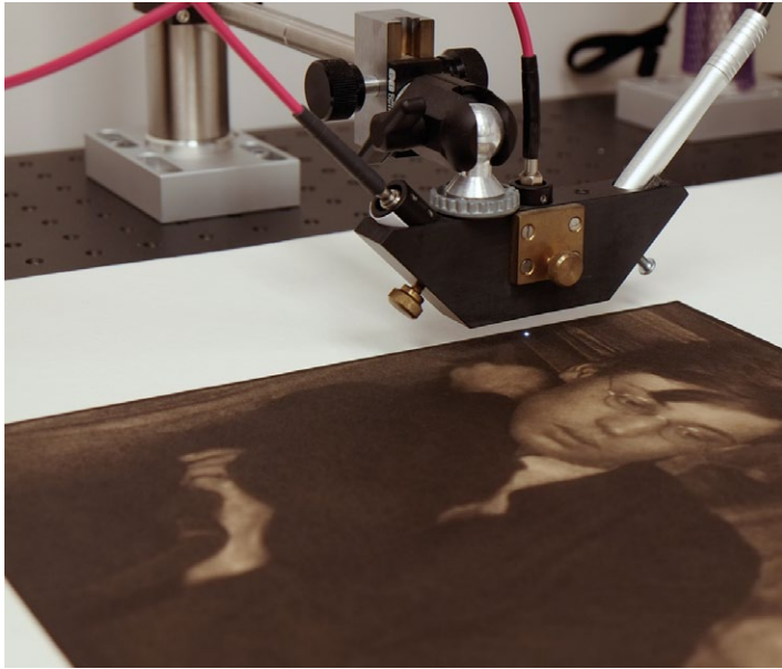
Figure 2. Microfading tester measurement head, designed by the author in 2006. The head is held at approximately 1 cm from the surface being tested. Focused light from the illumination fiber optic can be seen at the edge of this gum dichromate over platinum print by Heinrich Kühn (fig. 20 in Andreas Gruber, “The Platinum Print Technology of the Austrian Pictorialist Heinrich Kühn,” in this volume). The collection fiber optic (red) and the digital endoscope (silver), which is used for accurately positioning the measurement head, are both at 45° to the illumination fiber optic.
