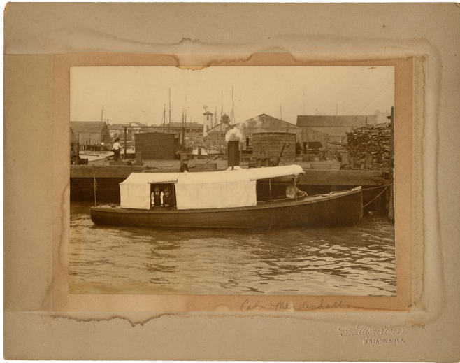
Figure 9. Photographer unknown, [ boat at dock 1 ], 1902. Matte collodion silver print toned with platinum, 11.3 × 16.2 cm. This is the recto of the image of the mount shown in figure 4b, and it is shown after the first aging experiment, with the six test papers (see table 1). Aging conditions were 80°C and 65% RH for 4 weeks.
