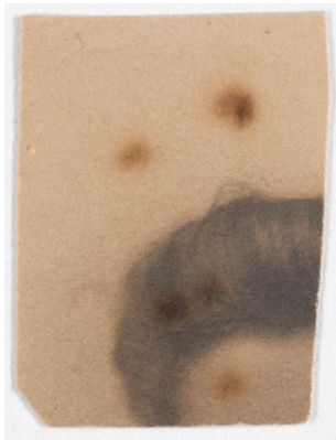
Figure 15. Detail of [ portrait of a woman ] (fig. 6) after aging in a capacitor-type assembly. The darkened spots that formed in the photograph were a result of aging; these exact areas had previously been analyzed by XPS.
