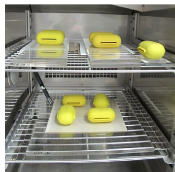
Figure 8. The environmental chamber used for accelerating-aging experiments. Initial aging conditions were 80°C and 65% RH for 4 weeks. Final aging conditions were 70°C and 65% RH for 6 weeks.
