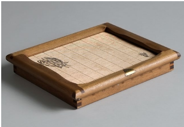
Figure 3. Mold and deckle used in hand papermaking. National Gallery of Art, Paper Conservation Department. Copper wires aligned in parallel rows form a laid screen. Watermark and countermark designs are sewn to the screen at the corners.
