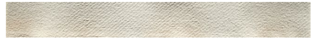
5b. In raking light. The diagonal texture is imparted by the weave of the drying felt.
