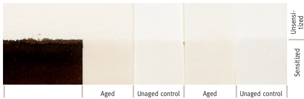
Figure 12. Platinum print exhibiting a noticeable sensitizer stain, prepared at the National Gallery of Art. The paper was sensitized partway up the paper, leaving a border of unsensitized paper at the top. The print was masked on the right side and fully exposed on the left. After processing, a faint difference between the sensitized and unsensitized areas can be observed. After accelerated aging, these regions are more pronounced.
