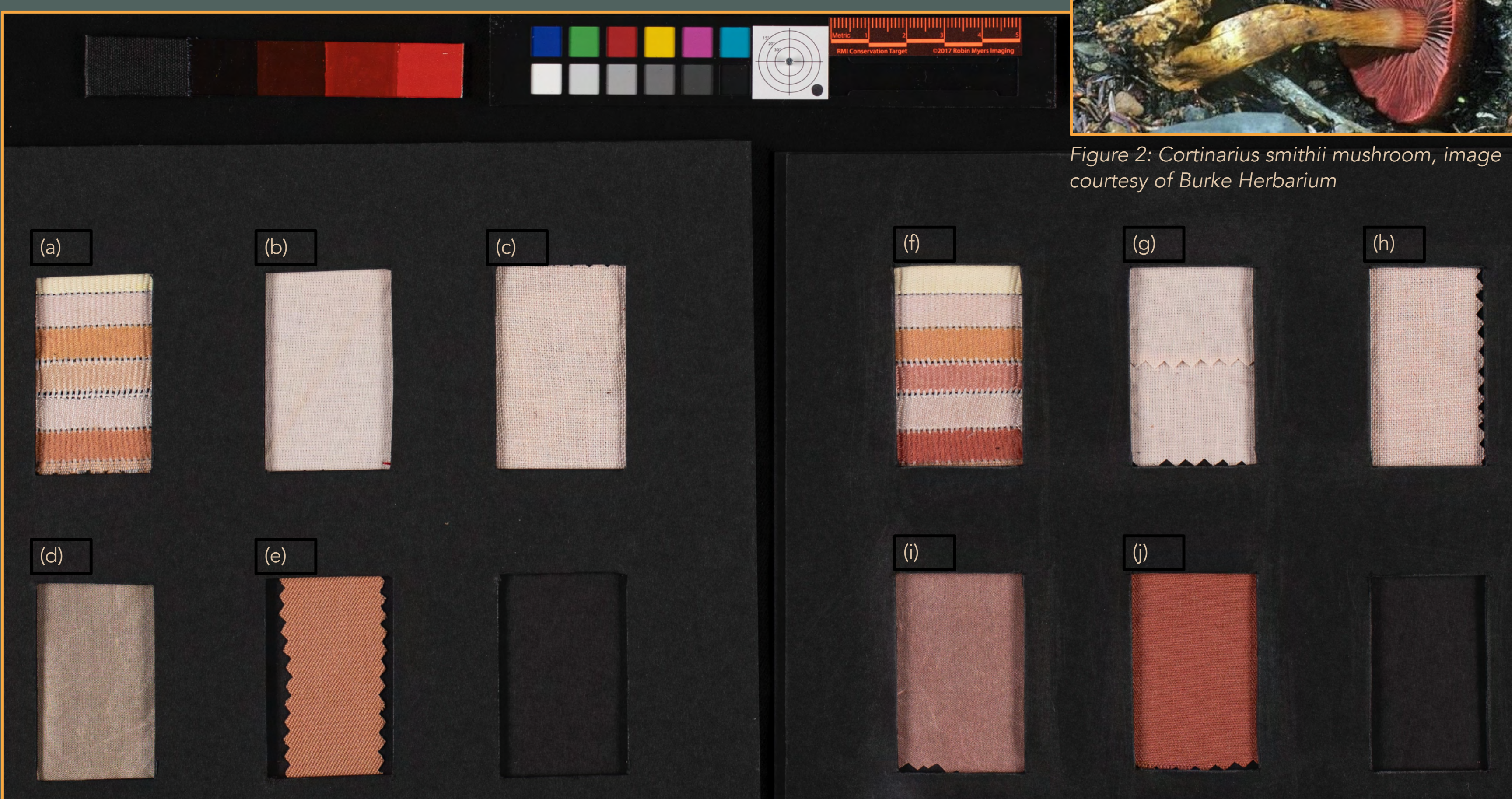
Figure 3: VIS image of Cortinarius smithii and semisanguineus dyed samples (unmordanted set on left, mordanted set on right). Unmordanted (a) Test Fabrics MMF 10A (bands top to bottom: acetate, cotton, nylon, polyester, acrylic, and wool); (b) cotton; (c) linen; (d) silk; (e) wool. Mordanted (f) Test Fabrics MMF 10A (bands as in (a)); (g) cotton; (h) linen; (i) silk; (j) wool.
