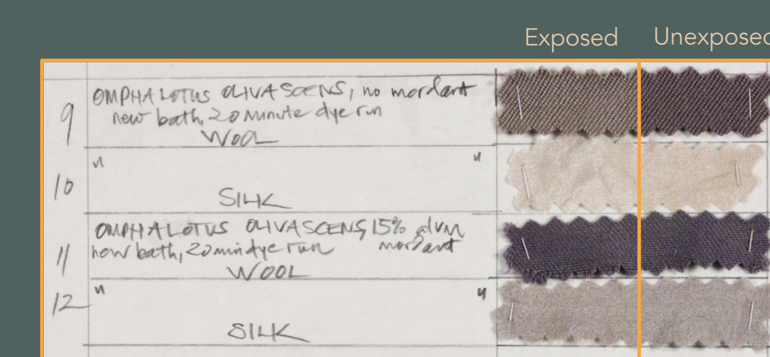
Figure 9: Omphalotus olivascens after aging, VIS; the lower two samples were mordanted with alum and exhibit much less fading than the unmordanted top two samples.
