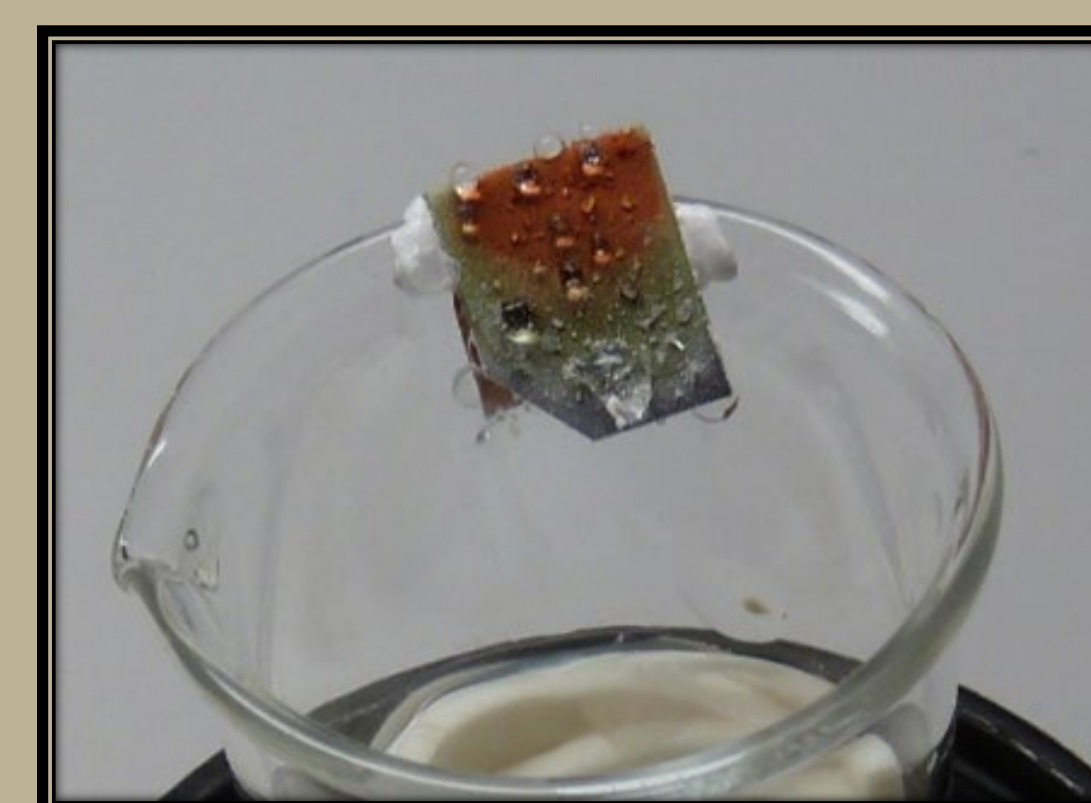
Failure of a lead coupon from a sample of PVAc cured 3 days, exhibiting layers of black, red and green corrosion products covering the entire surface, liquid droplets, surface delamination, and dense white extrusions adhering the coupon to the rim of the jar. Photo Cindy Connelly Ryan
