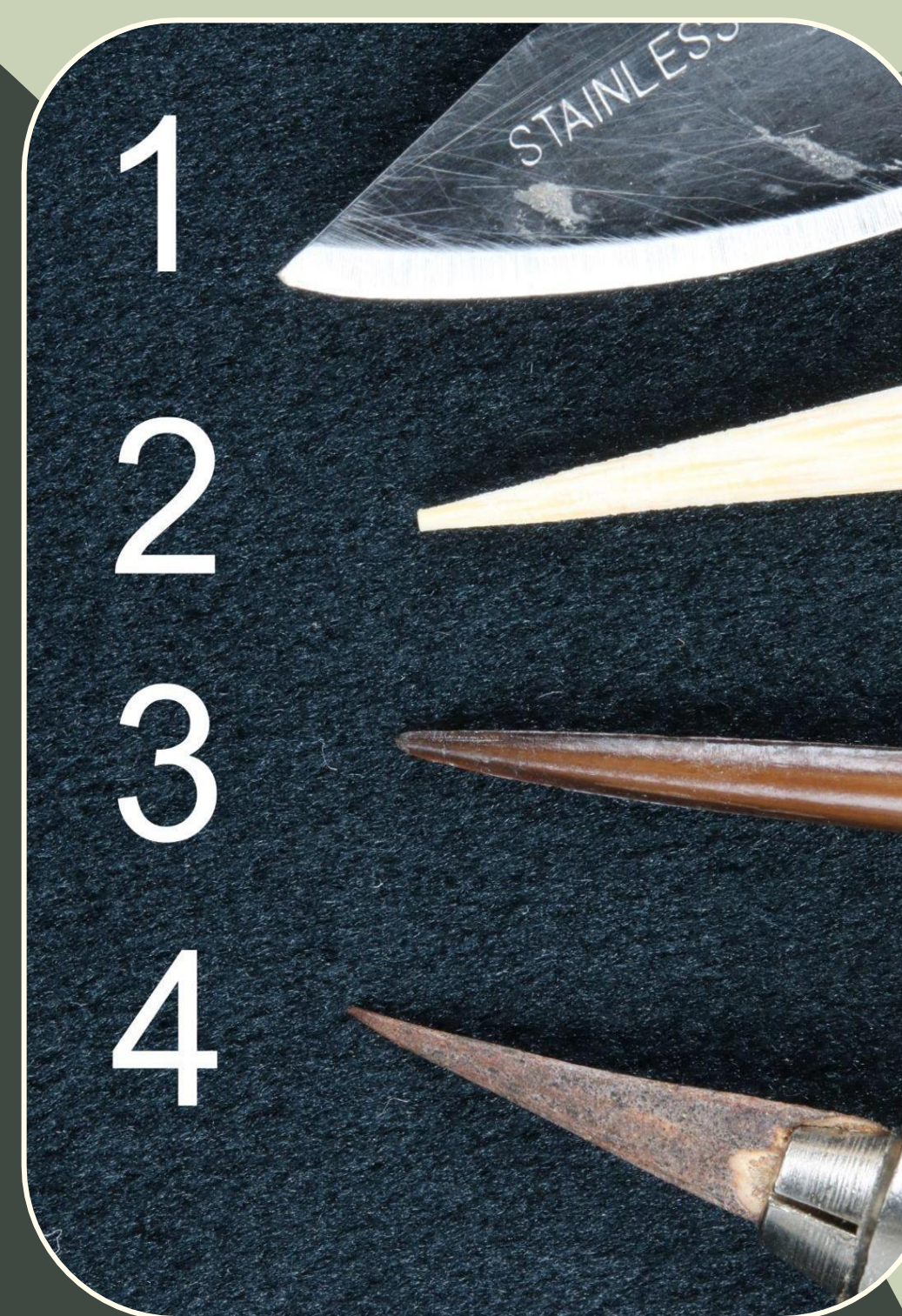
Common cleaning tools: 1) scalpel 2) bamboo skewer 3) porcupine quill 4) black locust thorn
