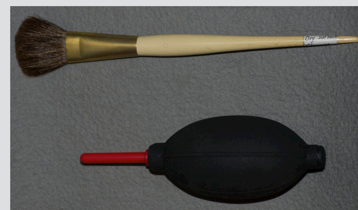
Tools used to test adhesion of flakes
