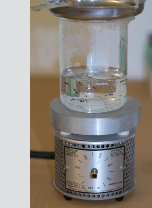
Boiling in NaOH
