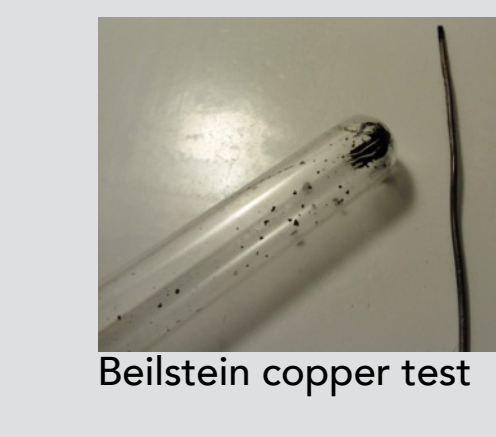
Beilstein copper test
