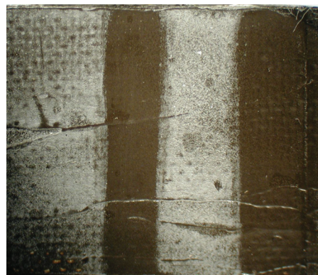
Figure 8. Close-up of raw umber paintout after treatment with naphtha followed by multiwax; the number of crystals is greatly reduced after treatment.
