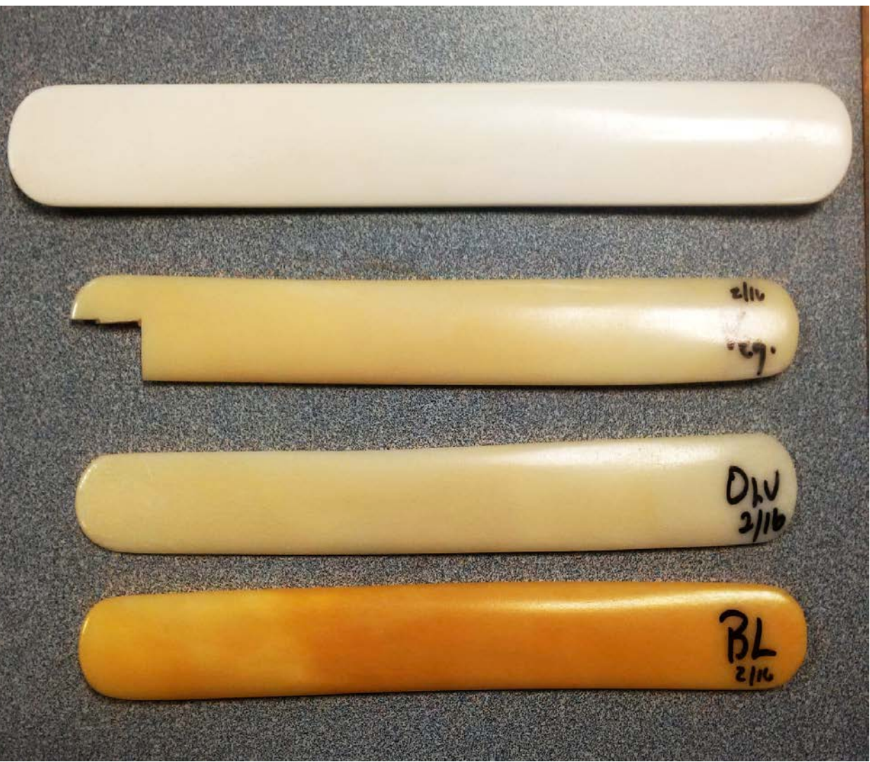
From top to bottom: • Natural, untreated cow bone, • Cow bone aged with vegetable oil, • Cow bone aged with olive oil, • Cow bone aged with boiled linseed oil. Note: The cut-off piece was used for testing.
