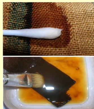
Fig. 6. Dry cleaning process
